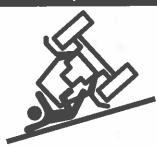
Narrow front end tractors can be unstable when equipped with a front end loader and can rollover. Use extreme caution when operating a narrow front end tractor equipped with a loader.
